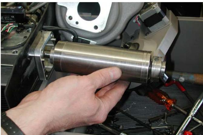
9. To replace the cartridge, slide into block, but do not tighten set screws.
