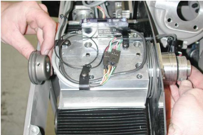
Remove the pulley and pull the cartridge out through the front of the block.
