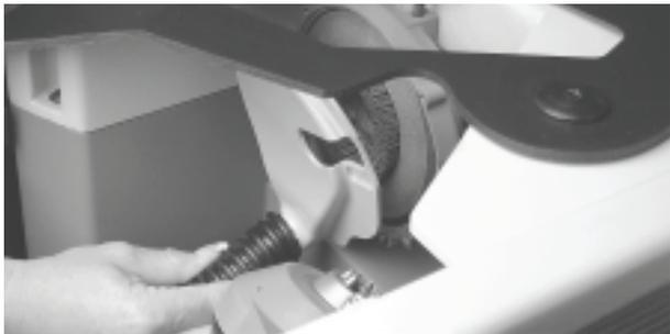
5. Insert spindle lock pin through access hole located on top of wheel guard casting.
