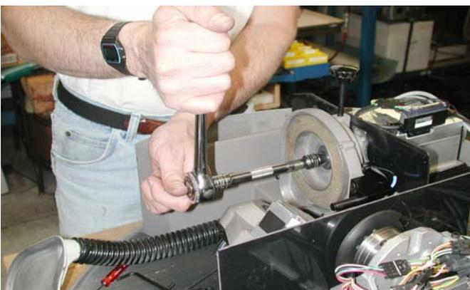
5. Remove the 4, 4mm screws holding the wheel casting in place.
