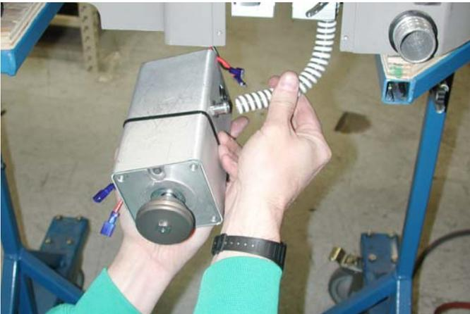
10. To replace the motor assembly, the machine must be in the belt change position.
