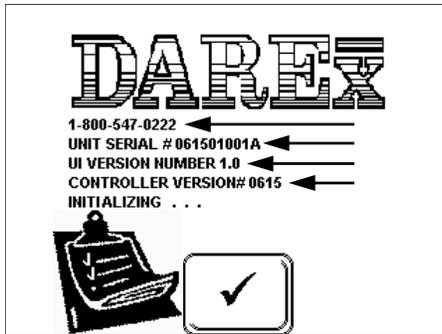
The initialization screen displays important information. On the first line you will find the Darex toll free phone number, the 2<sup>nd</sup> line displays the machine serial #. The 3<sup>rd</sup> line
