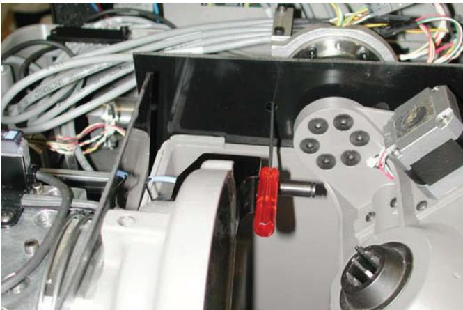
3. Swing the dust shield up or down to access the two 2mm screws securing the sensor.
