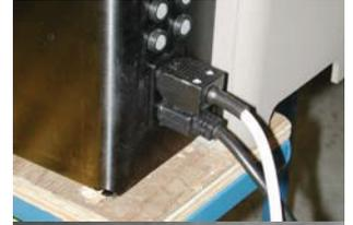
2. Located on the right side of the machine is the ON/OFF rocker switch. To power up machine, push rocker switch up.
