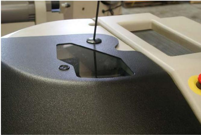
2. Remove the door support cover and lift the top cover.
