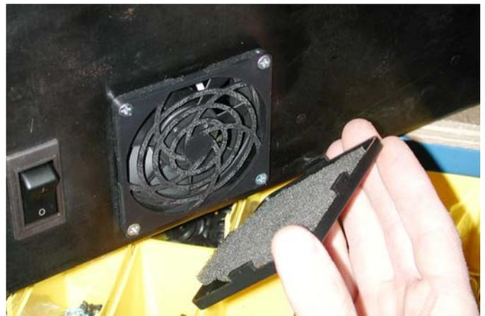
6. Using a nut driver to hold the nuts inside the panel, remove the 4 screws holding the fan in place. The front cover comes off and the fan can be removed from the inside along with the aluminum baffle.
