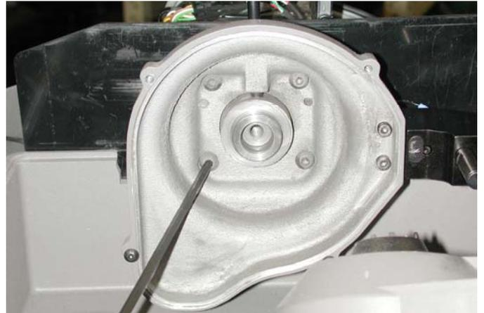
The casting is pinned to the cartridge block. With gentle pressure pull the casting from the block but do not disconnect any wires. It may be necessary to tap with a soft mallet. Carefully place the casting out of the way.
