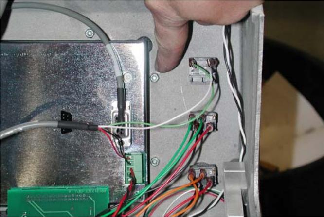
1. To replace the LCD, slip back through the front of the top cover. Hold in place with your hand and install acorn nuts just until one to two threads protrude past the surface of the nut. A thin wall ¼" socket is necessary for clearance.
