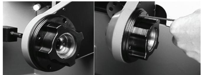
4. The chuck jaw assembly can now be removed through the back of the chuck spindle assembly.
