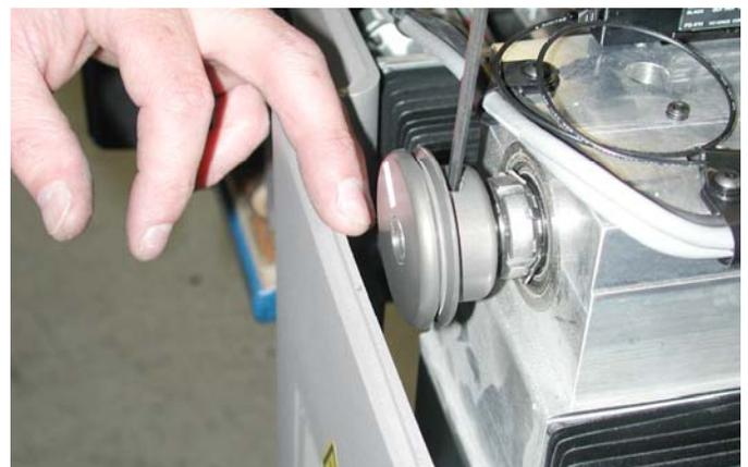
7. Loosen the 2, 3mm set screws in the top of the cartridge block that holds the cartridge in place.
