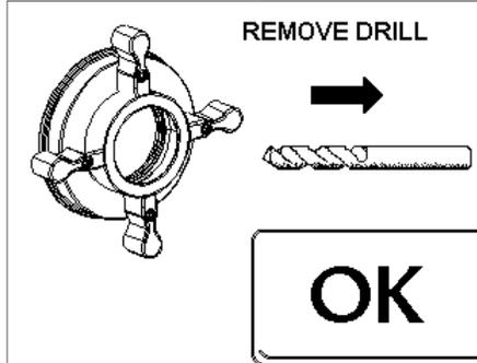
REMOVE DRILL ALARM - DRILL LEFT IN CHUCK Refer to information on page 63
