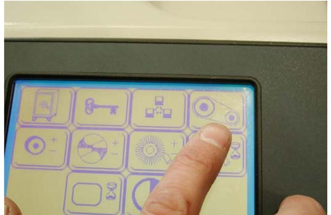
5. The X-Axis will move into the belt change position and stop. Shut the machine off and disconnect power source.
