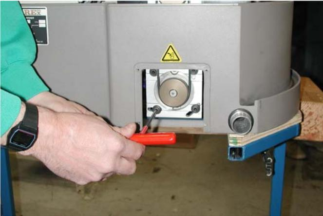
9. Slide the motor down the slotted bracket and out of the machine. Remove the cooling hose connected to the motor.
