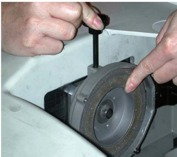
7. Using a 1/2 inch socket wrench, loosen wheel retainer bolt in the counterclockwise direction until wheel is free of the spindle.
