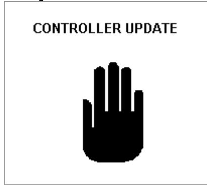
The Controller Update screen will flash on the screen and then the LCD screen will go dark.
