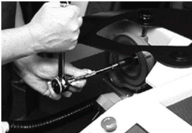
8. Repeat steps in reverse to install new wheel. Tighten to 12 lbs/per foot.
