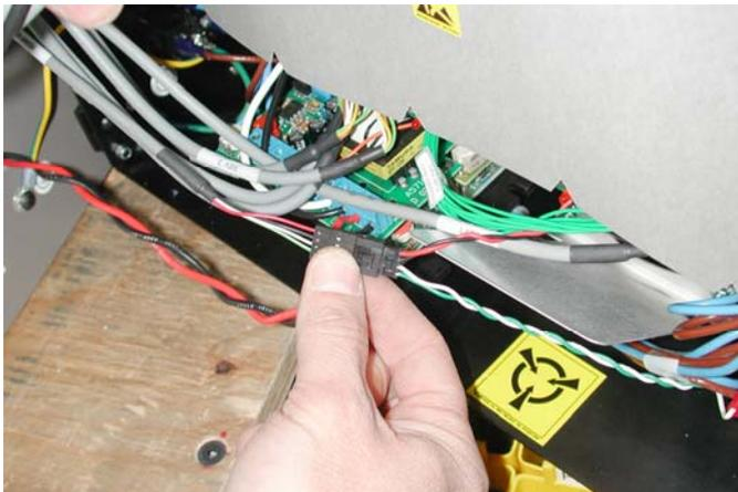
4. Note the white and green wires that go to the switch. Pull the 2 blade connectors from the switch.
