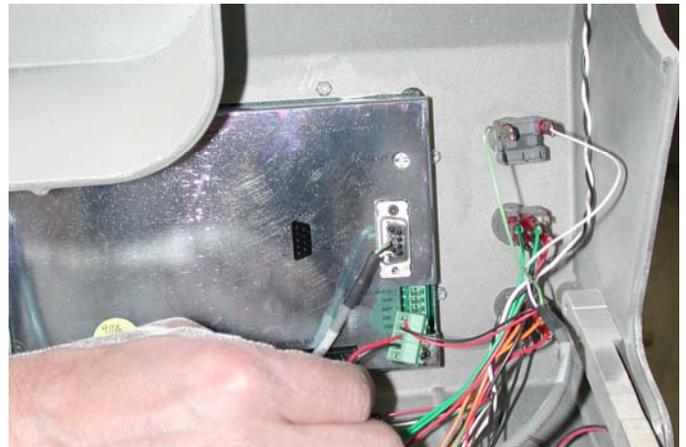
5. Remove the single screw on the RS232 connector and unplug from the LCD.
