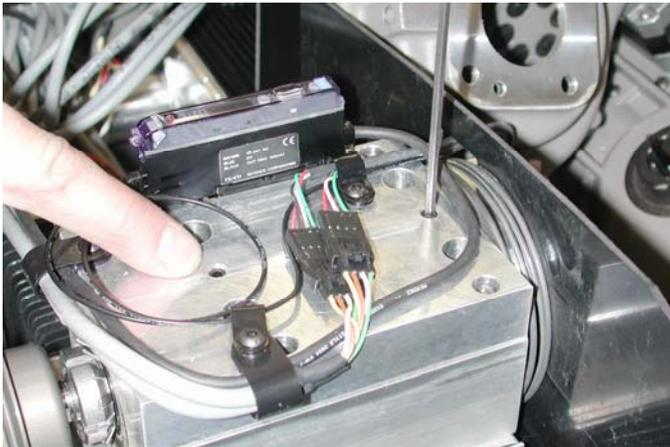
8. Slide the cartridge forward allowing enough room to remove the drive pulley.
