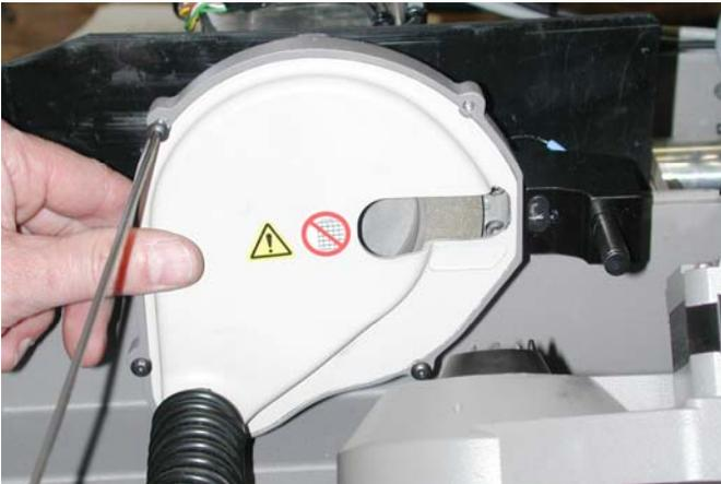
3. Slide the arbor lock pin through the hole in the wheel guard casting and rotate wheel until it engages.
