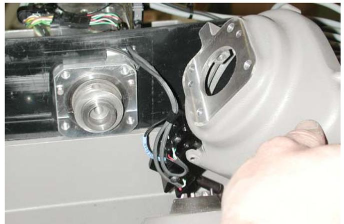
6. Loosen the 3mm set screw from the drive pulley, but do not remove.
