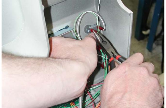
2. Connected to the switch is the switch block. Note the small key in the center left and to the right is a release clip. With a small blade screw driver reach down on the side of the clip and press inward while pulling up. The block will slide off.
