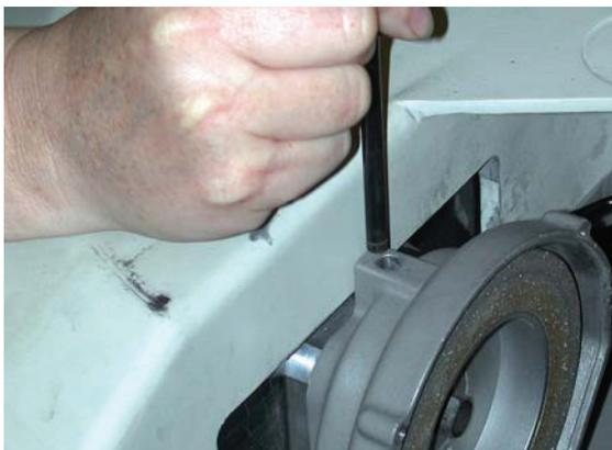
6. Rotate spindle until spindle lock pin engages.
