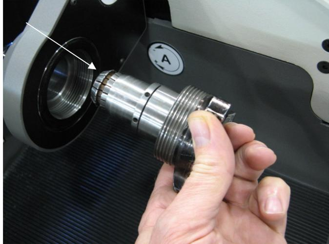
Install the Primary Knob into the Collet Chuck Spindle and tighten until contact of the collet is felt. Then back-off the knob  $\frac{1}{4}$  turn. Insert the drill through the collet as normal and then tighten the knob until snug.
