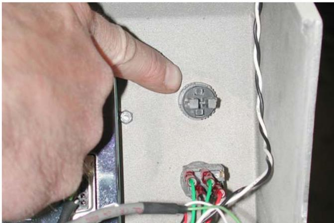
4. Slip the new switch in place with the key to the left or inside of the casting and the clip to the right or wall side of the casting.
