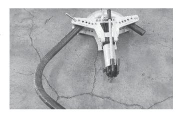
Before using the machine (pumping either pistons or retracting ram) open bleed/filler cap (as shown at right) a turn to allow air to escape or enter the hydraulic unit.
