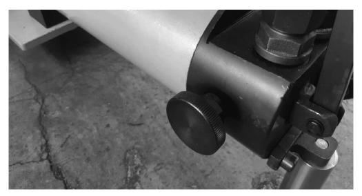
Open the top frame and fit the correct former for the pipe being bent. Fit the pipe being bent and close top frame. Fit the Bobbin and Bobbin pins into the corresponding holes for this size former (if  $1 \frac{1}{2}$ " former fitted the Bobbin and Bobbin pins must be fitted to the  $1 \frac{1}{2}$ " hole).
